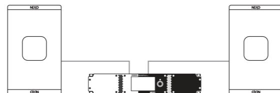
Active System: Stereo, 1 x P15 (Active) per side, powered by 1 x NXAMP4X2MK2
