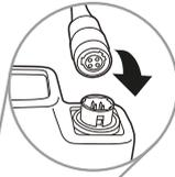
Locking 4-pin microphone connector for use with Audio-Technica cW-style wireless body-pack transmitters.
